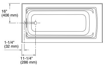
No change in measurements if connected with drain illustrated. (K-7272)
